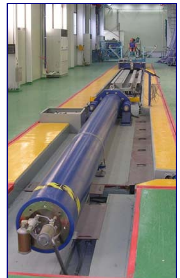
Delphi Korea 2.0MN ServoSled includes ServoSled controlled airbag squib firing system
